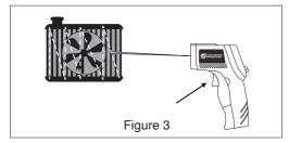
To find a hot spot, aim the thermometer outside of interest, and then scan across with an up and down motion until you locate the hot spot. (Figure 3)
