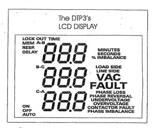
display the normal AB BC CA voltage pairs.
